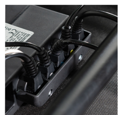
AFTER: CONTROL BOX CONNECTED WITH THE CAP
